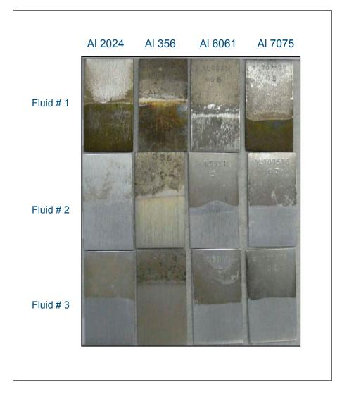
Figure 7 | An evaluation of the tendency for three fluids to stain four common aluminum alloys is shown. Fluids 2 and 3 are formulated with MEA, 3-amino-4-octanol and lower levels of TEA than what is used in Fluid 1, which also contains MEA. (*Courtesy of Dow Consumer & Industrial Solutions*)
