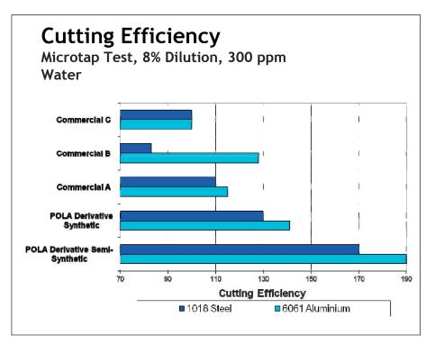
Figure 6 | Microtap test data shows that a POLA derivative can improve the performance of both a semisynthetic and synthetic fluid on aluminum and steel alloys. (*Courtesy of Croda Inc.*)
