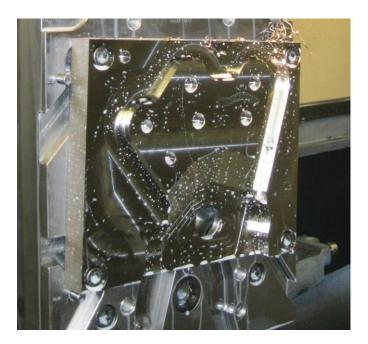
Figure 1 | A metal-removal operation on a titanium plate that is 12x12x2 inches thick is shown. (Courtesy of The Boeing Co.)
