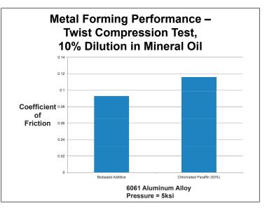
Figure 8 | A fluid formulated with 10 percent of a biobased boundary lubricity additive displays a superior coefficient of friction than a fluid formulated with 10 percent chlorinated paraffin in the Twist Compression Test run on a common aluminum alloy. (Courtesy of Croda Inc.)
